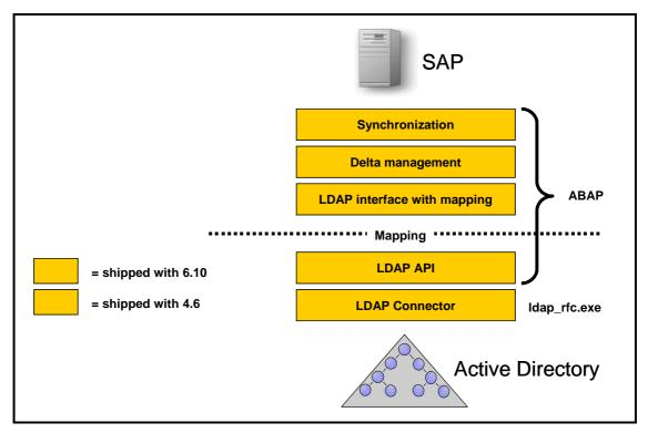
Figure 2 - Architecture of SAP LDAP Connector
