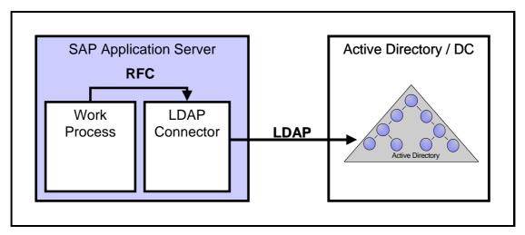
Figure 3 - Option a) LDAP Connector as part of the SAP application server
