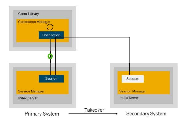
Per default the invisible takeover is deactivated. It can be activated with the following SAP HANA parameter setting:
